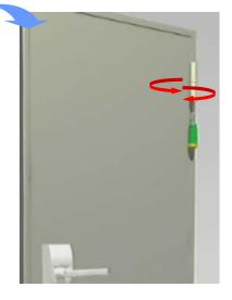
⑦ If door closing pattern is not good, control speed adjustment valve in the bottom of the product (at this time, remove fastened rubber band)
