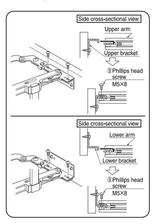
If the screws cannot be tightened downward when securing the upper door bracket, they can be tightened upward from under the joint. In that case, be sure to use the screw holes (inside the elliptical holes) in the upper door bracket.
