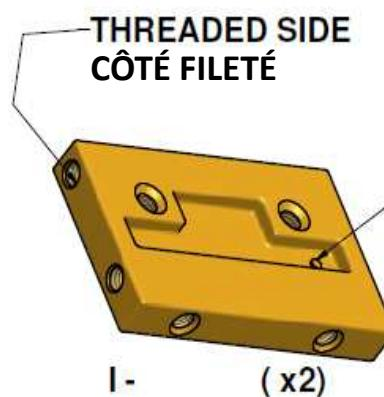
INSERT THE ZAMAK JOINTS (THREADED SIDE IN THE INSIDE OF THE SLIDES) AND FIX IT WITH THE INDICATED SCREWS.
