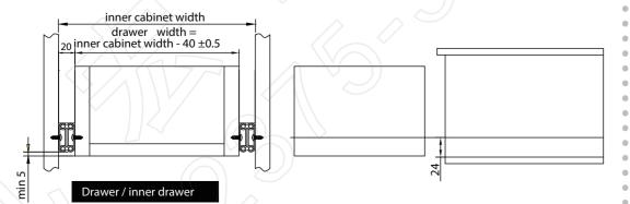
The bottom of drawer slides must be 5mm above the bottom of drawer to ensure correct function.
