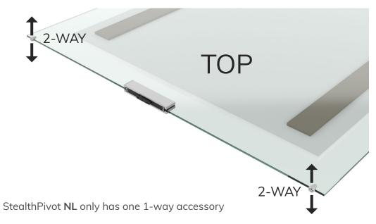
2-way + magnets can be mounted on both sides of the XL panel.
